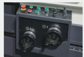
Manual operation box
